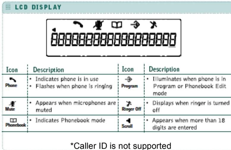
Each Conference Pod is equipped with an LCD display and uses Icons to assist in conference processing.
